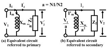
Figure 24.4: Equivalent circuits with  $X_m$
