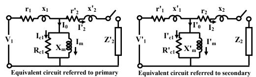
Figure 24.9: Exact Equivalent circuit referred to primary and secondary sides.
