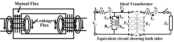
Figure 24.7: Leakage flux and their paths.
