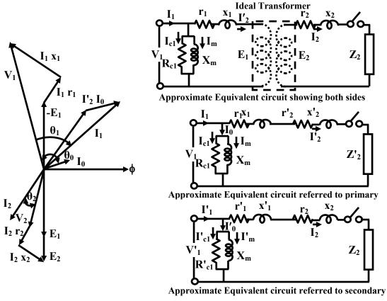
Figure 24.10: Phasor diagram of the transformer supplying lagging power factor load.
